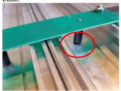
4. Remove the two nuts that line up with the holes in the circuit board, then finger tighten them onto the board to secure it to the bottom of the track. Do NOT over tighten as you may need to adjust the circuit board later in the process.
