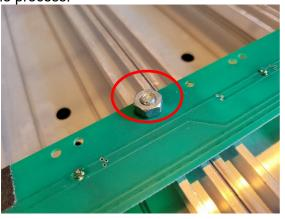
5. Carefully turn the track back over and make sure you can see the sensor through each of the four small holes in the track. Make adjustments as needed by reaching under the track and loosening and retightening the two nuts that keep the circuit board attached to the track. Finger tight is enough, do NOT over tighten.
