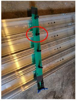
3. Align the circuit board so that the hoses line up with the smallest holes on the track. The connecting end of the circuit board will be on the right if you are looking toward the of the track.
