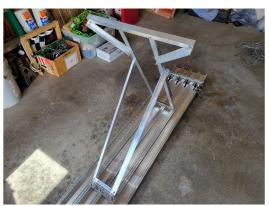
11. Carefully turn track A-1 over and set in place connecting to the curved piece A-2. Secure the remaining C-Clamps to keep the pieces together. Do NOT overtighten the C-Clamps to avoid damage to the track.
