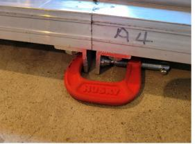
9. Connect the curved piece (A-2) to piece A-3 in the same manner as above. Use C-Clamps again by adjusting them first and placing them into position.
