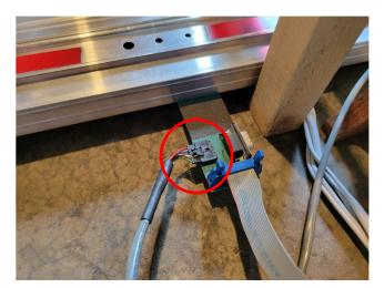
16. Connect the power supply to the starting gate. This will also power the Race Master finish line. You should see zeros above all 4 lanes.
