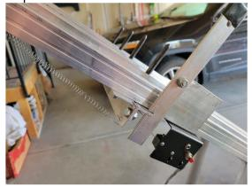
14. In order for the timer to work, the wire needs to sit under the drop gate such that the rotating switch is activated when the gate drops. Resetting the gate will also reset the switch. Make sure the wire moves freely with the drop gate.
